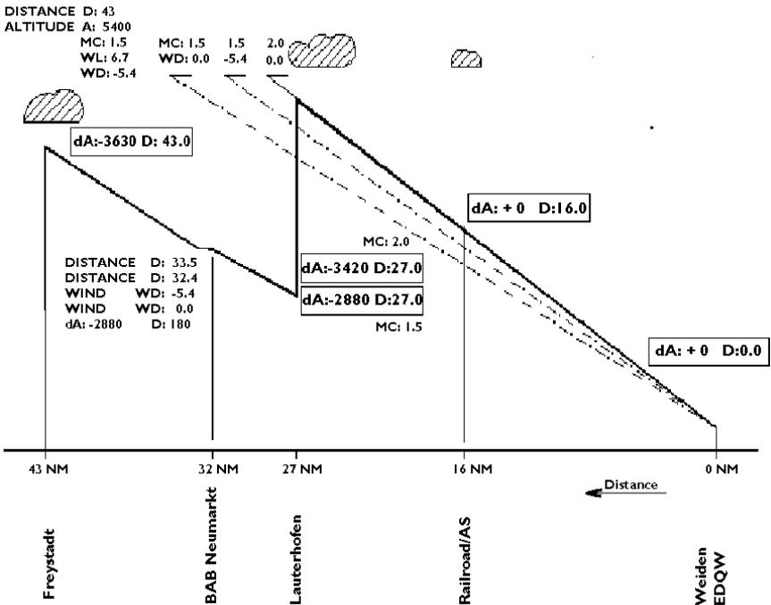
Where the 43 nm distance circle on the map crosses the canal, we start with the final glide. On the right bottom display quadrant already appears the final-glide distance  $\Delta E$  of 43.0 nm. This is identical with the remaining distance on  $d3 = D3 =$
